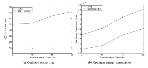
Fig. 5. Optimization results for  $\mathbf{P}_{min}^{eng}$  in underground environment as a function of volumetric water content.
