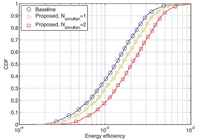
Fig. 4. Cumulative distribution of the energy efficiencies of 1000 random WUSNs with 5 nodes in 20 m  $\times$  20 m field.
