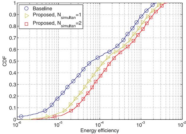
Fig. 5. Cumulative distribution of the energy efficiencies of 1000 random tunnel-based WUSNs with 5 nodes in 20 m  $\times$  20 m field.
