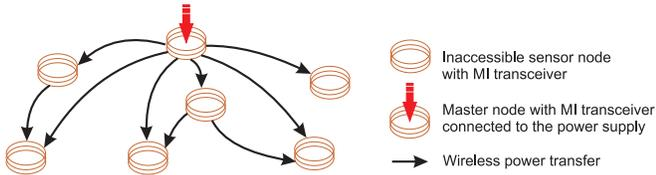
Fig. 1. Example of the network structure with a master node connected to the power supply.
