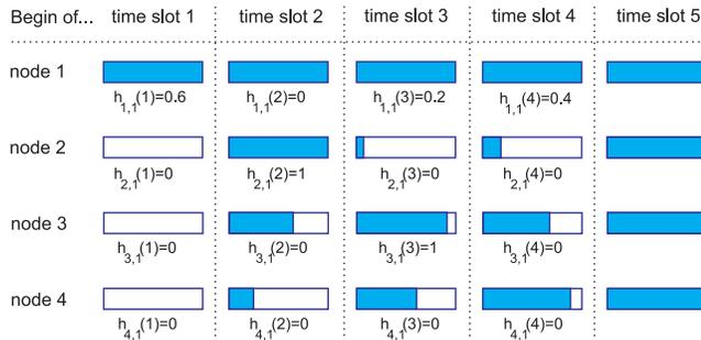
Fig. 3. Proposed scheduling for charging of three sensor nodes. Master node corresponds to node 1. Energy levels of nodes' batteries are shown.
