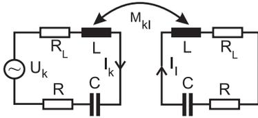
Fig. 2. Magnetic coupling between resonant circuits 'k' and 'l'.
