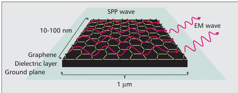
Figure 1. A graphene-based plasmonic THz Band antenna [10].
