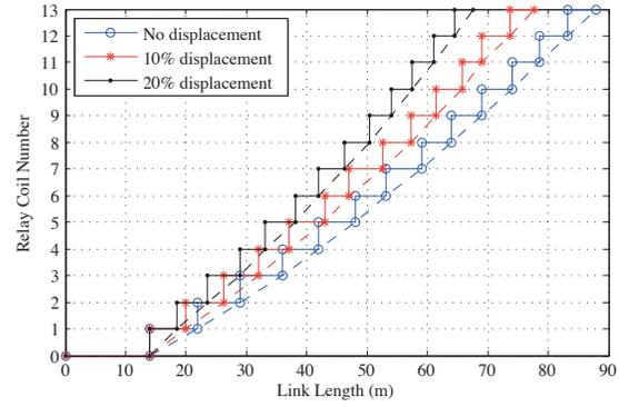
Fig. 3. Optimal relay coil number with different link length and displacement intensity.
