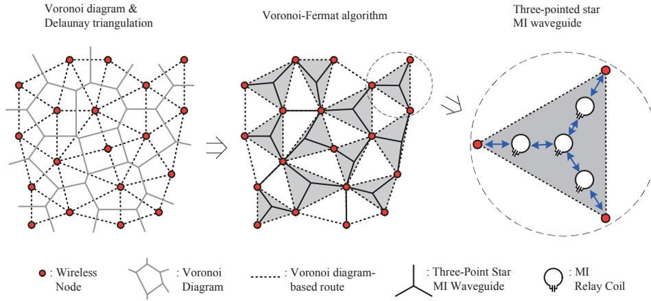
Fig. 4. The MI waveguide deployment using VF algorithm in the MI-based networks with random node distribution.
