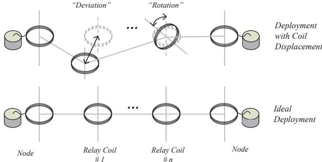
Fig. 2. Illustration of the possible relay coil displacements.
