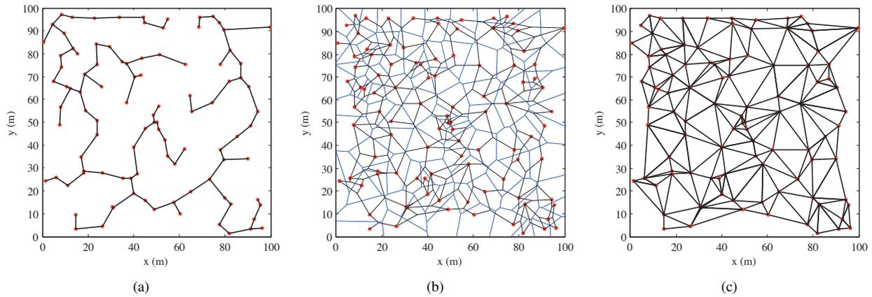
Fig. 6. The deployment results of (a) the MST algorithm, (b) the VF algorithm, and (c) the VF strategy without the Fermat improvement. (The red dots are the wireless nodes; the black lines represent the MI waveguides; and the blue cells are the Voronoi diagrams. 100 wireless nodes are uniformly distributed with of a spatial intensity  $\lambda_{rand} = 0.01 \text{ m}^{-2}$ .)
