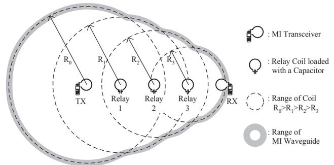
Fig. 1. The structure and the communication range of a MI waveguide.
