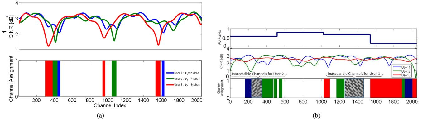
Fig. 6. Channel assignment behavior with (a) no existing PU activities and (b) different PU activity levels and inaccessible bands constraints.
