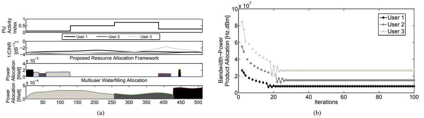
Fig. 7. (a) Resource allocation behavior at different levels of PU activities and (b) convergence of bandwidth-power allocation for each CR user.
