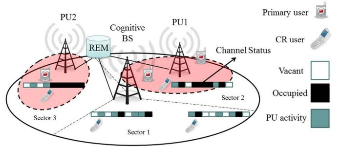
Fig. 1. Cognitive radio network deployment scenario. Radio Environment Maps (REM) is used for maintaining the records of PU activities
