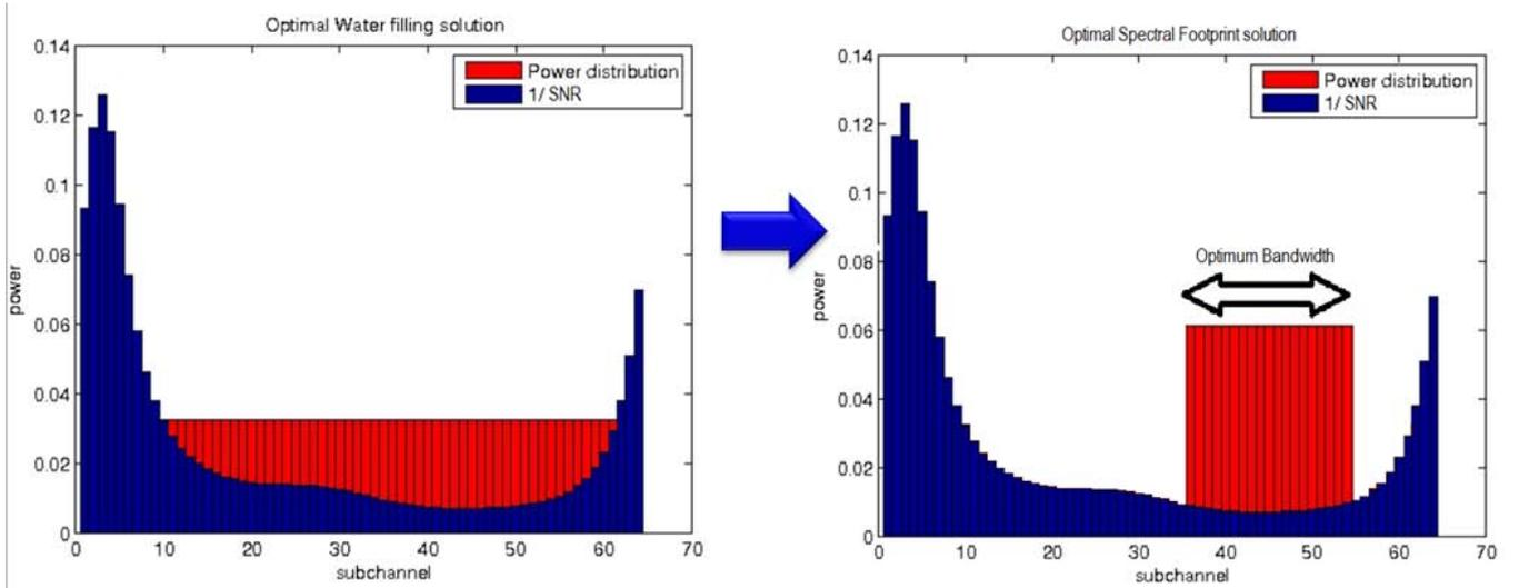
Fig. 2. Resource allocation using waterfilling and bandwidth-power product minimization.
