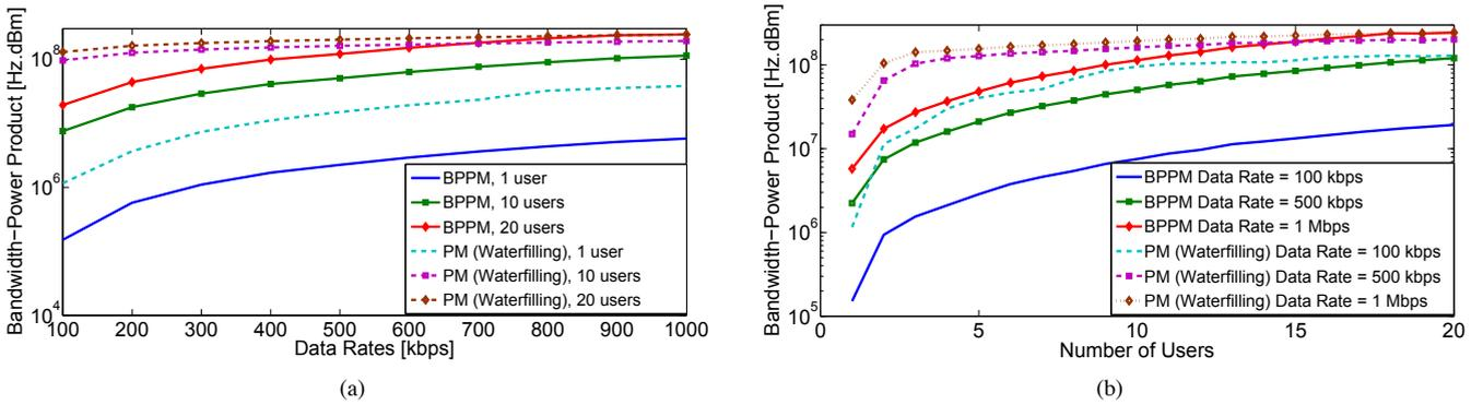
Fig. 8. Bandwidth-power product utilization of the proposed BPPM algorithm and the PM algorithm at different (a) data rates for 1, 10, and 20 users, and (b) number of users for data rate = 100 kbps, 500 kbps, and 1 Mbps.
