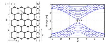
Fig. 2. Lattice structure of an AGNR (left) and energy band-structure an AGNR with  $N=18 \; (\Delta E=0.56 \; {\rm eV}).$
