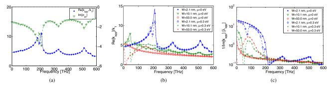
Fig. 5. (a) Real part of  $k_{spp}/k_1$  and imaginary part of  $\sigma_{yy}$  for an AGNR with W = 2.1 nm, (b) Real part of  $k_{spp}/k_1$  for different AGNR width W and chemical potential  $\mu$ , and (c) 1/e-amplitude decay propagation distance in terms of  $\lambda_{spp}$  for different AGNR width W and chemical potential  $\mu$  (T = 300 K).
