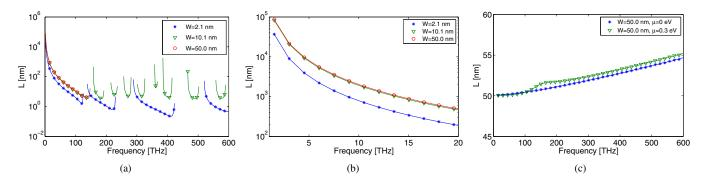
Fig. 6. (a) Antenna resonant length L for the fundamental TM mode (m = 1 in (27)) ( $\mu = 0.3$  eV)., (b) Antenna resonant length L for the fundamental TM mode in the Terahertz Band ( $\mu = 0.3$  eV), and (c) Antenna resonant length L for the fundamental TE mode (p = q = 1 in (28)) (T = 300 K).
