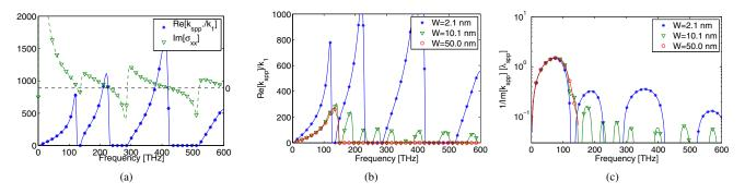
Fig. 4. (a) Real part of  $k_{spp}/k_1$  and imaginary part of  $\sigma_{xx}$  for an AGNR with W = 2.1 nm, (b) Real part of  $k_{spp}/k_1$  for different AGNR width, and (c) 1/*e*-amplitude decay propagation distance in terms of  $\lambda_{spp}$  for different AGNR width ( $\mu = 0.3$  eV, T = 300 K).
