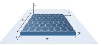
Fig. 1. A graphene-based plasmonic nano-patch antenna.
