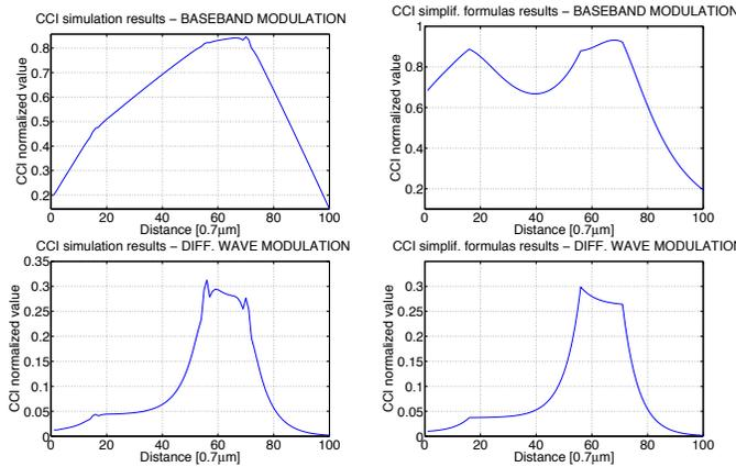
Fig. 4. The CCI values for the the baseband modulation scheme (upper) and the diffusion wave modulation scheme (lower) from the simulation (left) and from the simple formulas (right).
