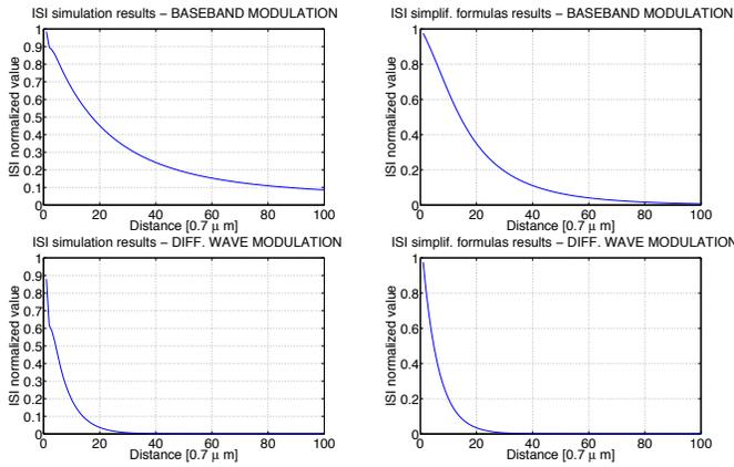
Fig. 3. The ISI values for the baseband modulation scheme (upper) and the diffusion wave modulation scheme (lower) from the simulation (left) and from the simple formulas (right).
