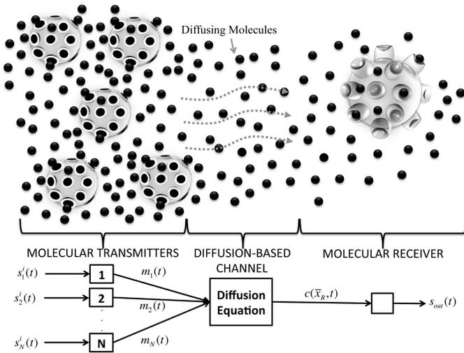
Fig. 1. Block scheme of the diffusion-based MC system considered in this paper.
