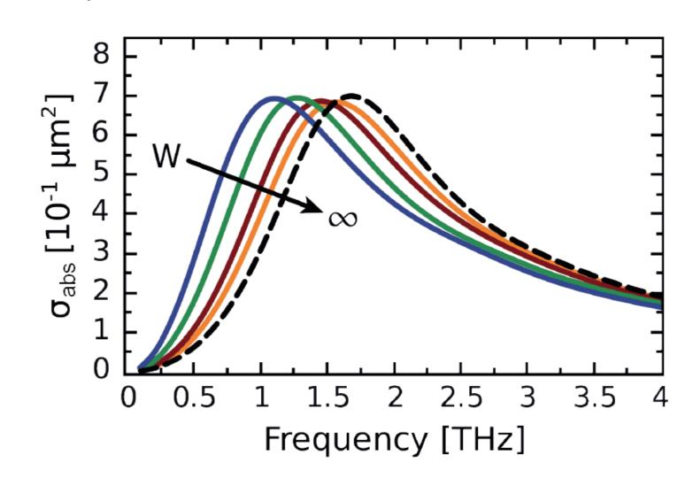
Dependence of the absorption cross section of a graphene-based nano-patch antenna as a function of its width. The antenna length is L = 5 μm. The plots correspond to infinite, 10 μm, 5 μm, 2 μm and 1 μm wide patches (right to left).
