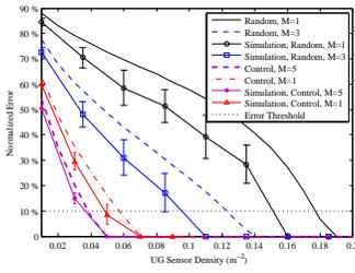
Fig. 2. Normalized monitoring error as a function of the sensor density.
