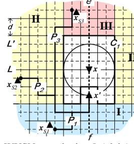
Fig. 1. Mapping the WUSN on a lattice  $L$  (plain) and its dual  $L'$  (dashed).
