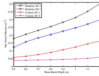
Fig. 4. Optimal sensor density as a function of the mean burial depth.
