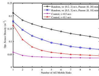
Fig. 3. Optimal sensor density as a function of the mobile sink number.
