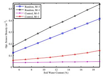
Fig. 5. Optimal sensor density as a function of the soil water content.
