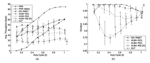
Fig. 8. (a) Average throughput and (b) average goodput versus duty cycle for different values of  $\xi_{Th}$ .
