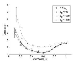
Fig. 7. Average latency versus duty cycle for different values of  $\xi_{Th}$ .
