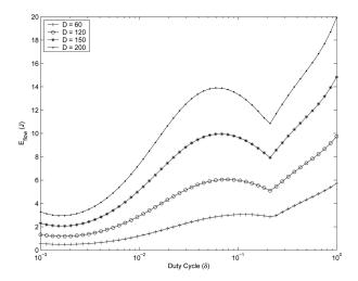
Fig. 4. Average energy consumption versus duty cycle for different values of  $\mathcal{D}.$
