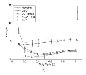
Fig. 10. (a) Average hop count and (b) average latency versus duty cycle for layered protocol suites and XLP.
