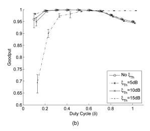
Fig. 6. (a) Average throughput and (b) average goodput versus duty cycle for different values of  $\xi_{Th}$ .
