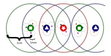
Fig. 3. BN example. The color and symbol of each node indicates the receiver attractant they emit and the circle around them their area of influence. (For interpretation of the references to colour in this figure legend, the reader is referred to the web version of this article.)
