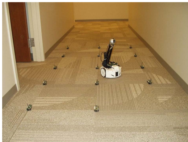
Fig. 9. GARCIA deployed on the sensor testbed. It acts as a mobile sink and can move to the area of interest for closer visual inspection. It can also coordinate with other actors and has built-in collision avoidance capability.
