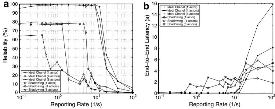
Fig. 9. Measurements with wireless realistic channel: (a) reliability versus reporting rate, (b) end-to-end latency versus reporting rate.
