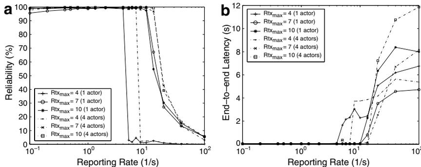
Fig. 8. (a) Reliability, and (b) end-to-end latency versus reporting rate for different values of retransmission limit,  $Rtx_{max}$ .
