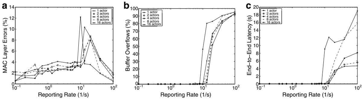
Fig. 3. (a) MAC layer errors, (b) buffer overflows, and (c) end-to-end latency versus reporting rate for different number of actors.
