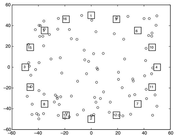
Fig. 1. Sample topology used in the simulations. The circles represent the sensors while the squares represent the actors.
