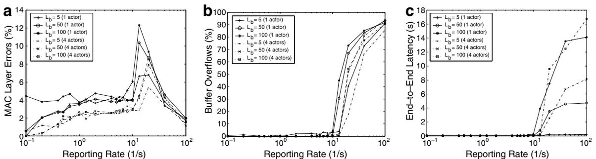
Fig. 7. (a) MAC layer errors, (b) buffer overflows, and (c) end-to-end latency versus reporting rate for different values of buffer length.
