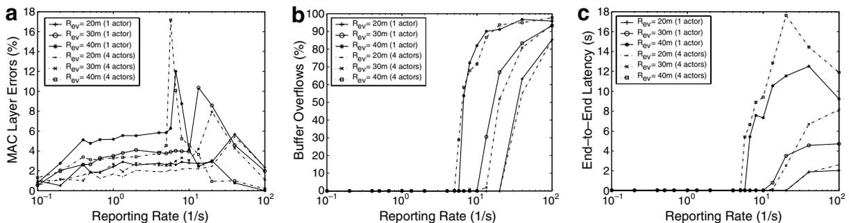
Fig. 5. (a) MAC layer errors, (b) buffer overflows, and (c) end-to-end latency versus reporting rate for different values of event radius,  $R_{ev}$ .
