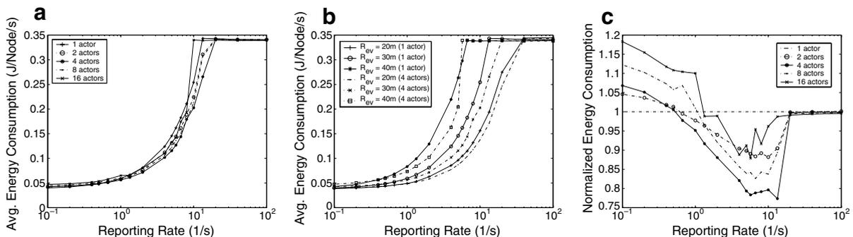
Fig. 10. (a) Average energy consumption per node for different number of actors, (b) average energy consumption per node for different event radius, and (c) average energy consumption normalized to the energy consumption of a single actor scenario.
