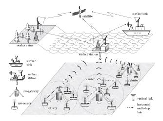
Figure 1: 2D Underwater Sensor Networks
