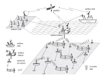
Figure 3: 3D Underwater Sensor Networks with AUVs
