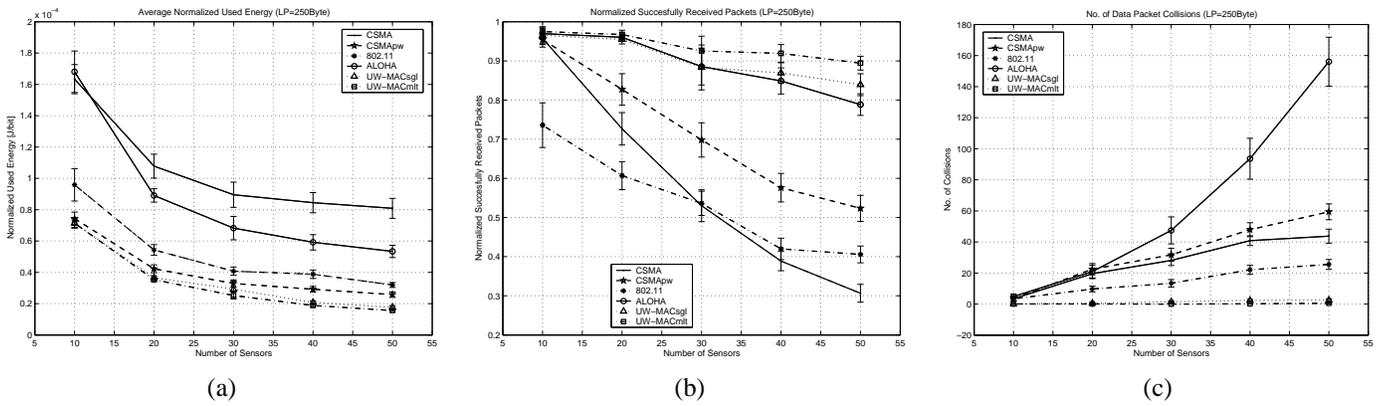
Fig. 3. **2D Deep Water UW-ASNs.** (a): Average normalized used energy vs. number of sensors; (b): Normalized successfully received packets vs. number of sensors; (c): Number of data packet collisions vs. number of sensors
