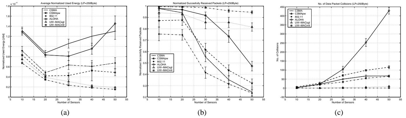
Fig. 5. **3D Shallow Water UW-ASNs.** (a): Average normalized used energy vs. number of sensors; (b): Normalized successfully received packets vs. number of sensors; (c): Number of data packet collisions vs. number of sensors
