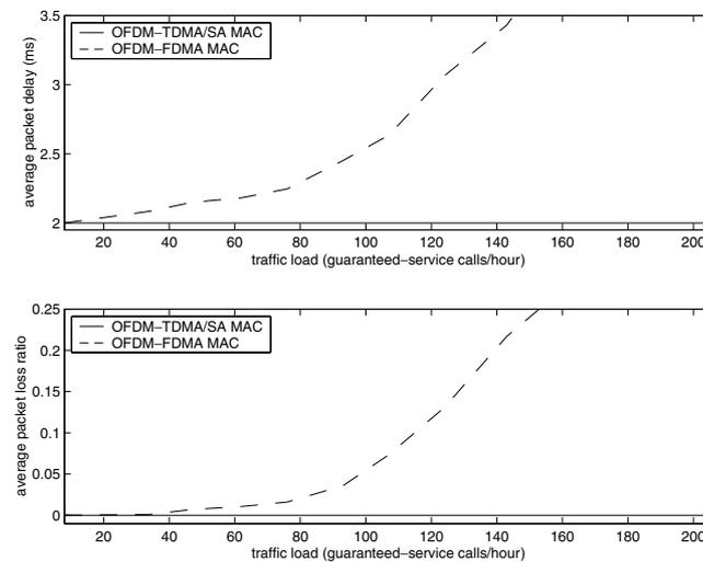
Figure 12. The average packet delay and packet loss ratio of guaranteed service.
