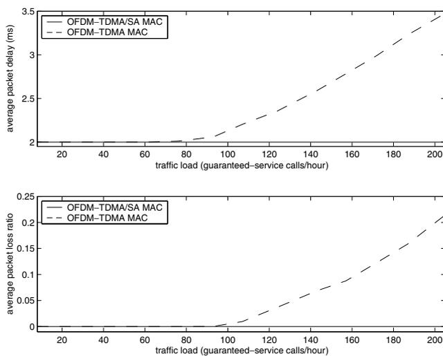
Figure 8. The average packet delay and packet loss ratio of guaranteed service.
