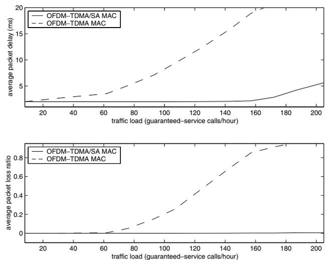
Figure 9. The average packet delay and packet loss ratio of controlled-load services.
