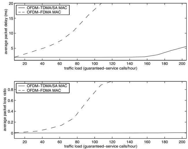
Figure 13. The average packet delay and packet loss ratio of controlled-load services.
