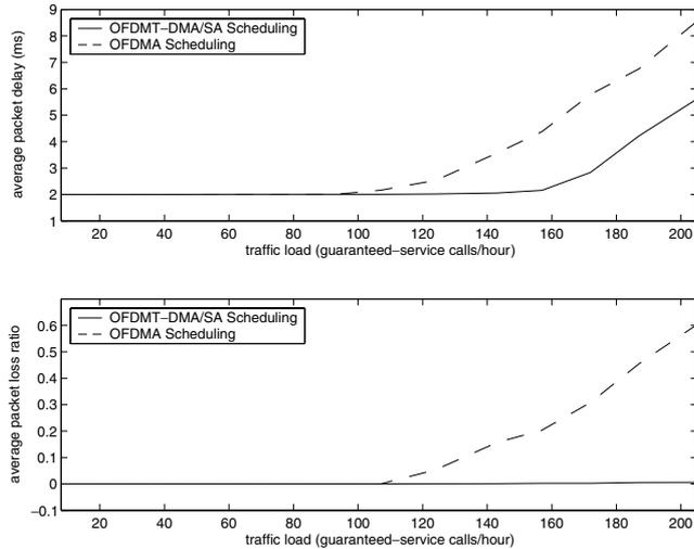
Figure 5. The average packet delay and packet loss ratio of controlled-load services.
