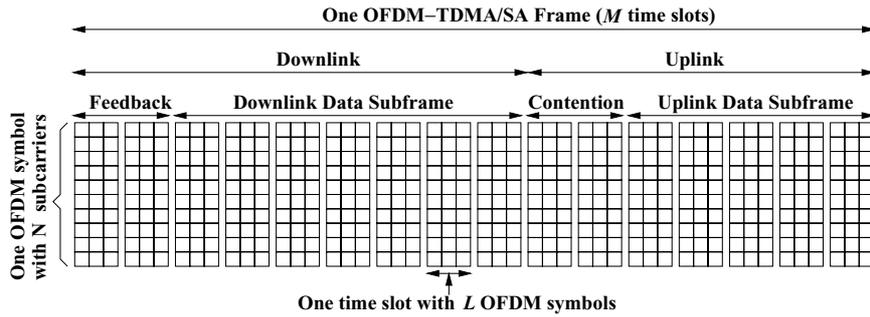
Figure 1. OFDM-TDMA/SA frame structure.
