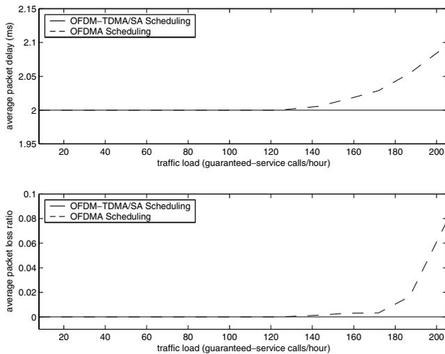
Figure 4. The average packet delay and packet loss ratio of guaranteed service.
