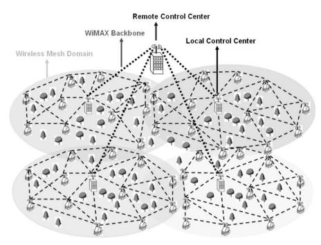
Fig. 7. An illustration of hybrid network architecture using WiMAX and wireless mesh networks.
