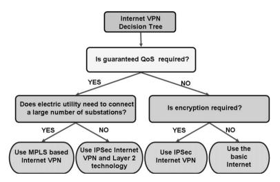
Fig. 4. A basic Internet VPN decision tree for electric system automation.
