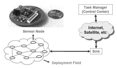
Fig. 5. An illustrated architecture of wireless sensor networks.
