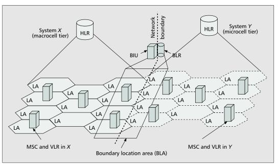
**Figure 5.** The boundary location area (BLA) and boundary location register (BLR).
