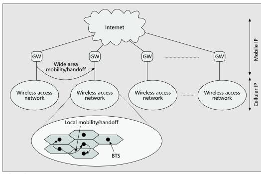
Figure 4. Cellular IP architecture.
