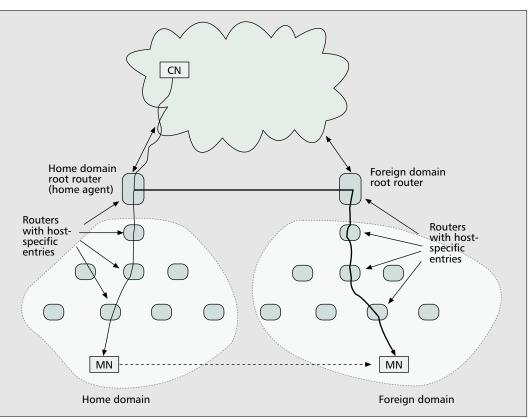
Figure 4. The network architecture of HAWAII.
