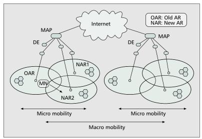
**Figure 6.** *The architecture of the S-MIP scheme.*
