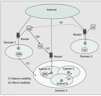
**Figure 1.** *Mobile IP architecture.*
