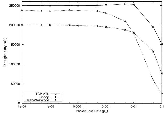
Fig. 6. Throughput comparison of TCP-ATL, Snoop, and TCP-Westwood for  $d_w = 10$  ms and varying  $p_w$ .
