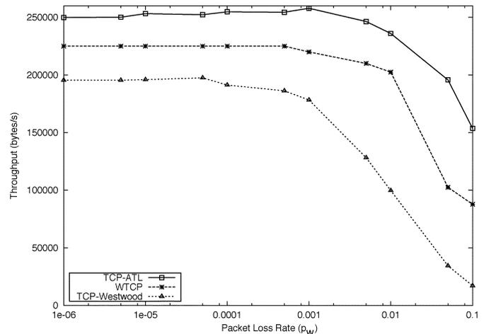
Fig. 7. Throughput comparison of TCP-ATL, WTCP, and TCP-Westwood for  $d_w = 50$  ms and varying  $p_w$ .
