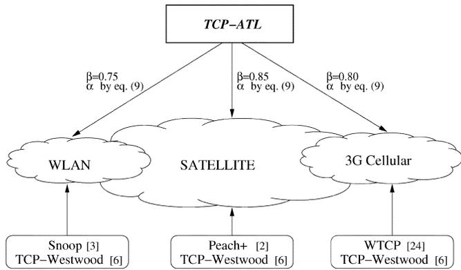
Fig. 5. Unified and adaptive TCP-ATL protocol instead of using different transport protocols that are specifically designed for different wireless architectures.
