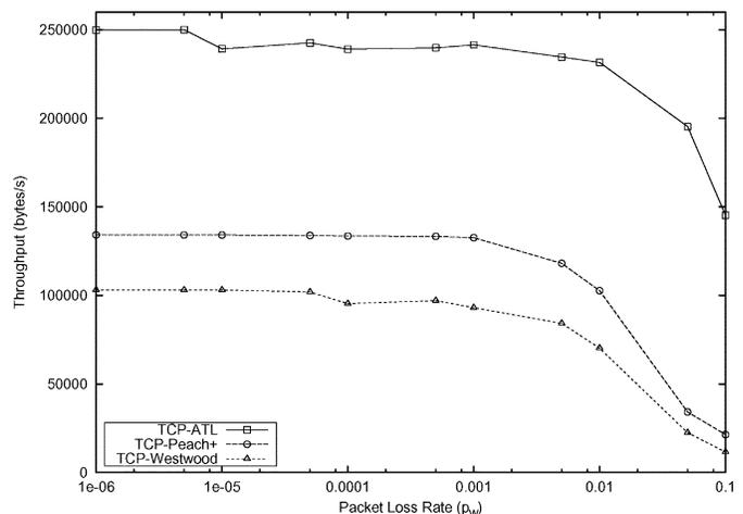
Fig. 8. Throughput comparison of TCP-ATL, TCP-Westwood, and TCP-Peach+ for  $d_w = 150$  ms and varying  $p_w$ .
