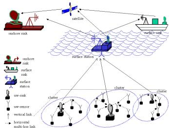
Fig. 1. Architecture for 2D Underwater Sensor Networks.
