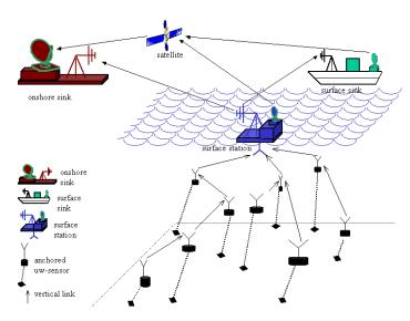
Fig. 2. Architecture for 3D Underwater Sensor Networks.
