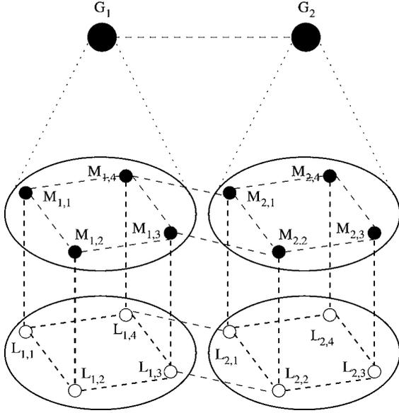
Figure 1. The architecture of the hierarchical satellite network.
