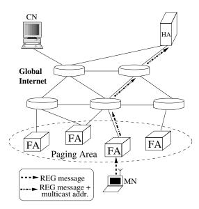
Fig. 2. Procedure of location registration.
