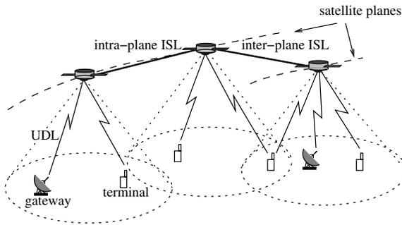
Fig. 1. Satellite network architecture.
