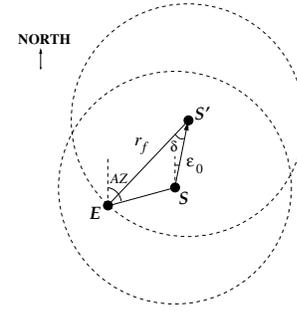
Fig. 2. Calculation of the remaining coverage time of  $S$  toward  $E$ .
