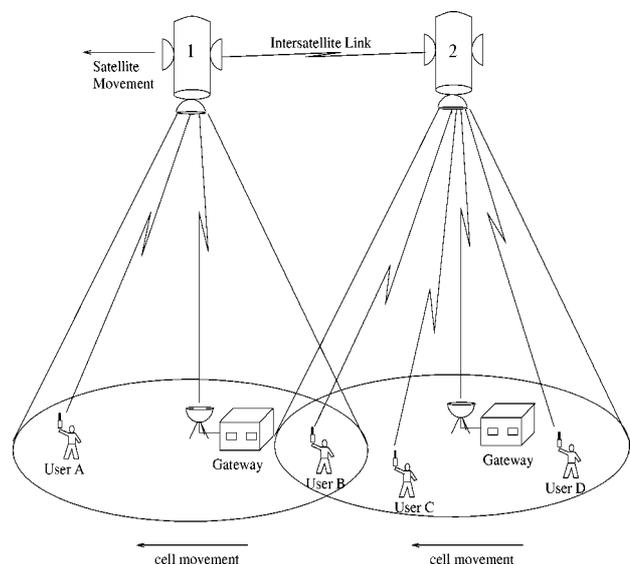
Figure 1. Wireless communication via LEO satellite network.
