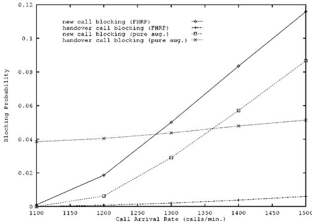
Figure 10. New call and handover blocking probabilities vs. call arrival rate for static, FHRP and pure augmentation networks.
