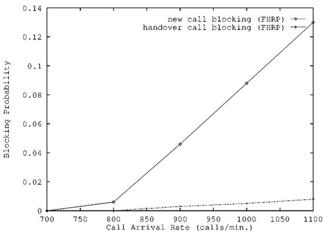
Figure 13. New call and handover blocking probabilities vs. call arrival rate for heterogeneous case.
