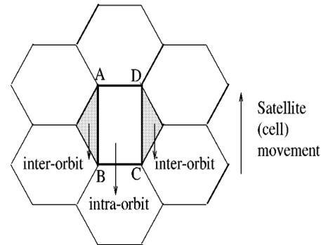
Figure 8. Inter- and intraorbit handover in augmentation algorithm.
