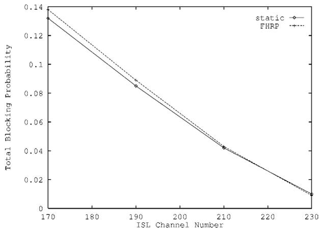
Figure 12. ISL blocking probabilities vs. number of ISL channels for heterogeneous case.
