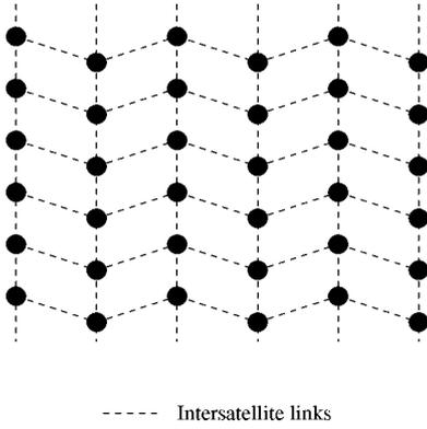
Figure 4. Intersatellite links between adjacent LEO satellites.
