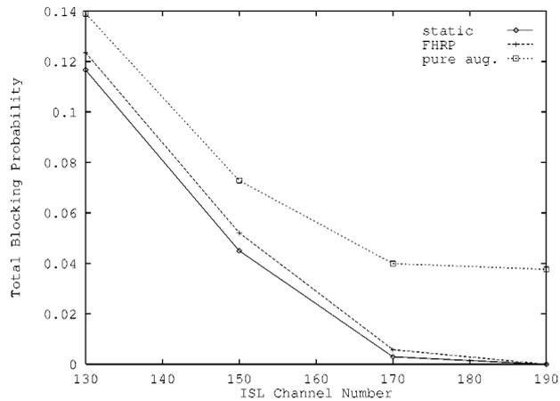
Figure 11. ISL blocking probabilities vs. number of ISL channels.
