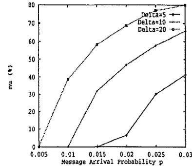
Figure 6: Percentage of Dropped Messages in the Single-VLA Scenario (40 MBSs, 200 MTs,  $D = 2$ , MBS mobility=1/time unit, MT mobility=2/time unit)
