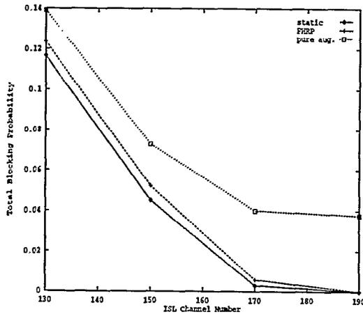
Figure 11: ISL Blocking Probabilities vs. Number of ISL Channels.
