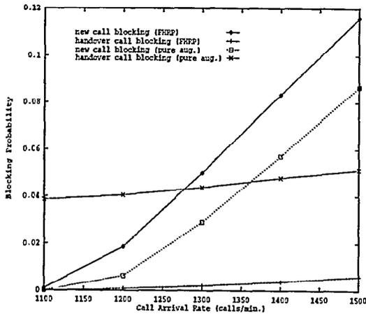
Figure 10: New Call and Handover Blocking Probabilities vs. Call Arrival Rate for Static, FHRP and Pure Augmentation Networks.
