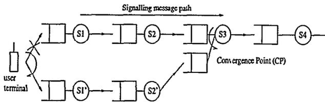
Figure 8: In-sequence Cell Delivery Algorithm.
