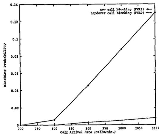
Figure 13: New Call and Handover Blocking Probabilities vs. Call Arrival Rate for Heterogeneous Case.
