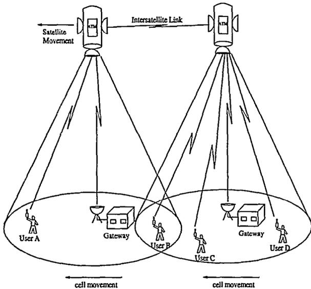
Figure 1: Wireless Communication via Satellite ATM Network.
