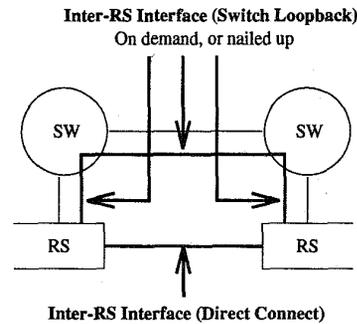
Figure 2: IRI Transmission Alternative
