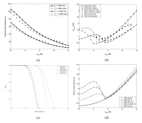
Fig. 3. (a) Average hop distance and (b) average energy consumption of a flow versus  $\psi_{Th}$ . (c) End-to-end PER versus  $\psi_{Th}$  and (d) average end-to-end latency versus  $\psi_{Th}$  (MicaZ).
