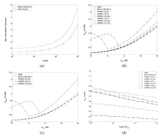
Fig. 7. (a) Maximum normalized taxonomy versus traffic load,  $\lambda$ . Average energy consumption versus  $\psi_{Th}$  for hybrid ARQ (b) Type I and (c) Type II and (d) average energy consumption versus target end-to-end PER (MicaZ).
