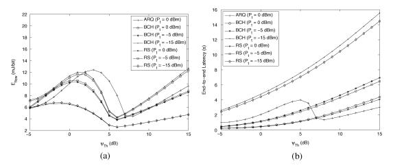
Fig. 5. (a) Average energy consumption of a flow and (b) average end-to-end latency versus  $\psi_{Th}$  for different values of transmit power (Mica2).
