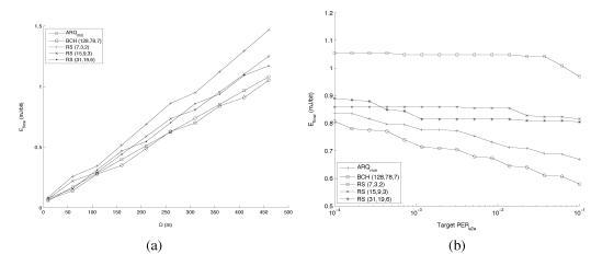
Fig. 6. Average energy consumption versus (a) end-to-end distance and (b) target end-to-end PER for MicaZ nodes.
