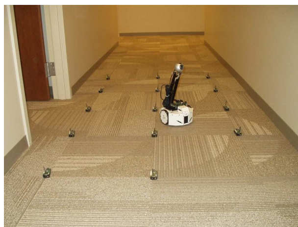
Fig. 9. GARCIA deployed on the sensor testbed. It acts as a mobile sink and can move to the area of interest for closer visual inspection. It can also coordinate with other actors and has built-in collision avoidance capability.
