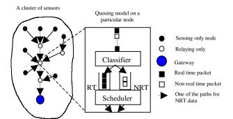
Figure 2. Queuing model in cluster-based sensor network
