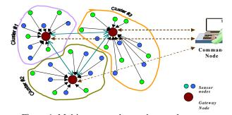
Figure 1. Multi-gateway clustered network sensors node is located within the communication range of all the sensors of its cluster. Clustering the sensor network is
